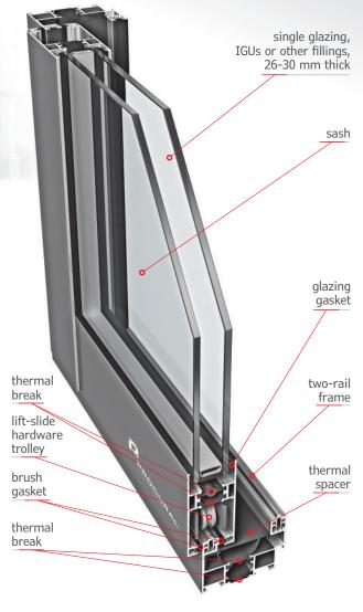
An insulated aluminium profile system designed for the construction of sliding windows and spatial constructions such as balcony and loggia structures
